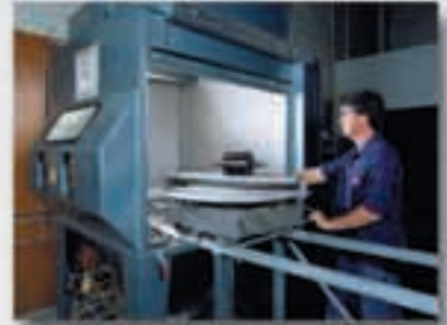
Beadblasting parts in final cleaning stage
