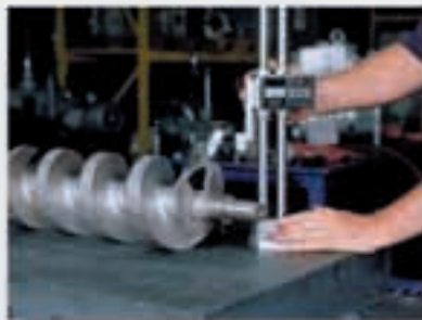
Measuring screw dimensions
